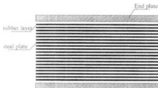
Fig. 1 Model of steel reinforced elastomeric isolator
